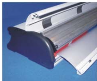
Place the banner cartridge into the base, ensure the cartridge rod is seated correctly into groove 1. Rotate the cartridge until the remaining rods are seated into grooves 2 and 3
